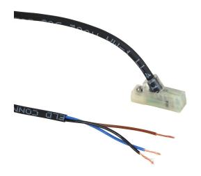
NITRA cylinder switch, rectangular, PNP, N.O. output, 5-28 VDC operating voltage, LED indication, 9.8ft (3.00m) 3-wire pigtail with wire leads, 45-degree cable entry, 6.5 x 3.2mm T-slot mount, for position sensing.
