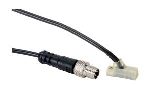
NITRA cylinder switch, rectangular, NPN, N.O. output, 5-28 VDC operating voltage, LED indication, 0.5ft (0.15m) cable with 3-pin M8 snap-fit connector, 45-degree cable entry, 6.5 x 3.2mm T-slot mount, for position sensing.
