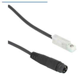
NITRA cylinder switch, dovetail, PNP, N.O. output, 5-28 VDC operating voltage, LED indication, 0.5ft (0.15m) cable with 3-pin M8 snap-fit connector, straight cable entry, 1/4in 60 degree dovetail slot mount, for position sensing.
