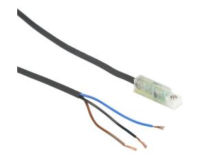
NITRA cylinder switch, dovetail, PNP, N.O. output, 5-28 VDC operating voltage, LED indication, 9.8ft (3.00m) 3-wire pigtail with wire leads, straight cable entry, 1/4in 60 degree dovetail slot mount, for position sensing.
