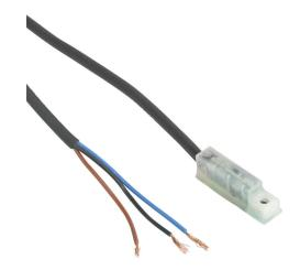
NITRA cylinder switch, dovetail, NPN, N.O. output, 5-28 VDC operating voltage, LED indication, 9.8ft (3.00m) 3-wire pigtail with wire leads, straight cable entry, 1/4in 60 degree dovetail slot mount, for position sensing.
