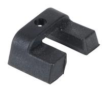
NITRA dovetail groove adapter, 14mm. For use with CPS9D cylinder position switch in a 60 degree dovetail slot.
