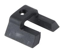
NITRA dovetail groove adapter, 12mm. For use with CPS9D cylinder position switch in a 60 degree dovetail slot.
