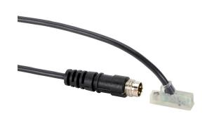
NITRA cylinder switch, dovetail, PNP, N.O. output, 5-28 VDC operating voltage, LED indication, 0.5ft (0.15m) cable with 3-pin M8 snap-fit connector, 45-degree cable entry, 1/4in 60 degree dovetail slot mount, for position sensing.
