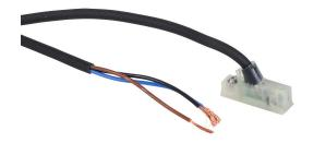
NITRA cylinder switch, dovetail, PNP, N.O. output, 5-28 VDC operating voltage, LED indication, 9.8ft (3.00m) 3-wire pigtail with wire leads, 45-degree cable entry, 1/4in 60 degree dovetail slot mount, for position sensing.
