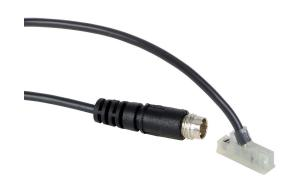
NITRA cylinder switch, dovetail, NPN, N.O. output, 5-28 VDC operating voltage, LED indication, 0.5ft (0.15m) cable with 3-pin M8 snap-fit connector, 45-degree cable entry, 1/4in 60 degree dovetail slot mount, for position sensing.
