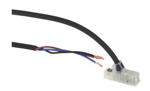
NITRA cylinder switch, dovetail, NPN, N.O. output, 5-28 VDC operating voltage, LED indication, 9.8ft (3.00m) 3-wire pigtail with wire leads, 45-degree cable entry, 1/4in 60 degree dovetail slot mount, for position sensing.
