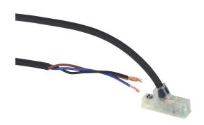
NITRA cylinder switch, dovetail, NPN, N.O. output, 5-28 VDC operating voltage, LED indication, 9.8ft (3.00m) 3-wire pigtail with wire leads, 1/4in 60 degree dovetail slot mount, for position sensing.
