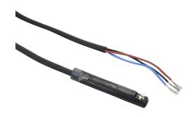
NITRA cylinder switch, round, NPN, N.O. output, 5-28 VDC operating voltage, LED indication, 9.8ft (3.00m) 3-wire pigtail with wire leads, straight cable entry, 4mm round slot mount, for position sensing.
