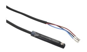
NITRA cylinder switch, round, NPN, N.O. output, 5-28 VDC operating voltage, LED indication, 9.8ft (3.00m) 3-wire pigtail with wire leads, 4mm round slot mount, for position sensing.
