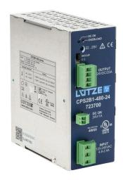
LUTZE CPS Ultra series switching power supply, 24 VDC @ 20A/480W, 120/240 VAC nominal input, 1-phase, enclosed, aluminum housing, 35mm DIN rail mount, screw terminals.
