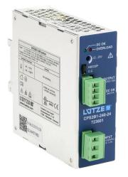
LUTZE CPS Ultra series switching power supply, 24 VDC @ 10A/240W, 120/240 VAC nominal input, 1-phase, enclosed, aluminum housing, 35mm DIN rail mount, screw terminals.
