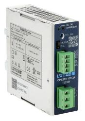
LUTZE CPS Ultra series switching power supply, 24 VDC @ 5A/120W, 120/240 VAC nominal input, 1-phase, enclosed, aluminum housing, 35mm DIN rail mount, screw terminals.
