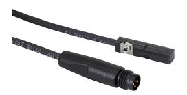
NITRA cylinder switch, square, PNP, N.C. output, 10-30 VDC operating voltage, LED indication, 0.3m (1ft) cable with 3-pin M8 snap-fit connector, straight cable entry, 5mm square T-slot mount, for position sensing.
