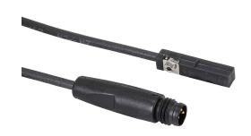
NITRA cylinder switch, square, PNP, N.O. output, 10-30 VDC operating voltage, LED indication, 0.3m (1ft) cable with 3-pin M8 snap-fit connector, straight cable entry, 5mm square T-slot mount, for position sensing.
