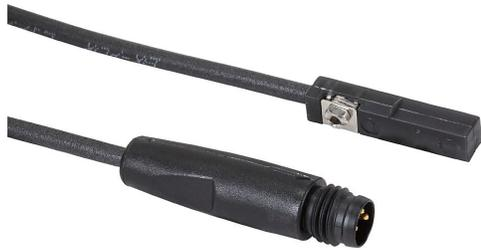
NITRA cylinder switch, square, PNP, N.O. output, 10-30 VDC operating voltage, LED indication, 0.3m (1ft) cable with 3-pin M8 snap-fit connector, straight cable entry, 5mm square T-slot mount, for position sensing.
