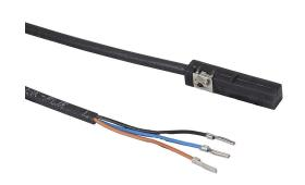
NITRA cylinder switch, square, PNP, N.O. output, 10-30 VDC operating voltage, LED indication, 2m (6.56ft) 3-wire pigtail with wire leads, 5mm square T-slot mount, for position sensing.
