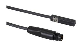
NITRA cylinder switch, square, NPN, N.O. output, 10-30 VDC operating voltage, LED indication, 0.3m (1ft) cable with 3-pin M8 snap-fit connector, 5mm square T-slot mount, for position sensing.
