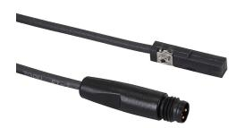
NITRA cylinder switch, square, NPN, N.O. output, 10-30 VDC operating voltage, LED indication, 0.3m (1ft) cable with 3-pin M8 snap-fit connector, straight cable entry, 5mm square T-slot mount, for position sensing.
