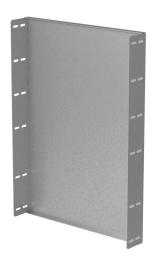
Quadritalia OK series modular mounting plate, 600 x 600mm (HxW), galvanized steel. For use with TMKxx6 inner frame in 600mm width enclosures.
