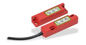
IDEM safety switch set, non-contact magnetic, (1) N.C. safety output(s), (1) N.O. monitoring output(s), plastic housing, 83 x 20mm, pigtail, 16.4ft/5m cable length.
