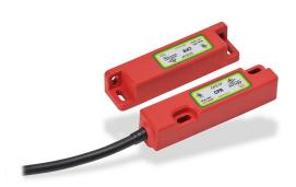
IDEM safety switch set, non-contact magnetic, (1) N.C. safety output(s), (1) N.O. monitoring output(s), plastic housing,  $83 \times 20$ mm, pigtail, 6.5ft/2m cable length.
