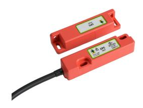
IDEM safety switch set, non-contact coded magnetic, (2) N.C. safety output(s), (1) N.O. monitoring output(s), plastic housing, 83 x 20mm, 8-pin M12 quick-disconnect, 9.8in/250mm cable length.
