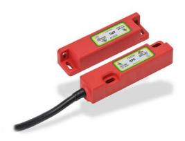
IDEM safety switch set, non-contact coded magnetic, (2) N.C. safety output(s), (1) N.O. monitoring output(s), plastic housing, 83  $\times$  20mm, pigtail, 16.4ft/5m cable length.
