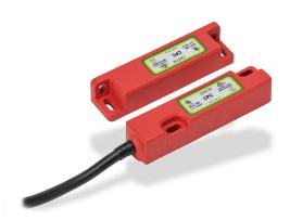
IDEM safety switch set, non-contact coded magnetic, (2) N.C. safety output(s), (1) N.O. monitoring output(s), plastic housing, 83 x 20mm, pigtail, 16.4ft/5m cable length.
