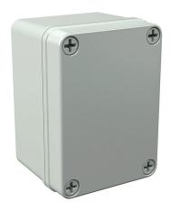
AttaBox Commander series pushbutton enclosure, blank cover, NEMA 1/3R/4X/6P/12, 4 x 3 x 2in (HxWxD), wall mount, polycarbonate, light gray, gloss finish, screw cover.
