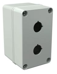
AttaBox Commander series pushbutton enclosure, 2 holes, 22mm, NEMA 1/3R/4X/6P/12, 5 x 3 x 3in (HxWxD), wall mount, polycarbonate, light gray, gloss finish, screw cover.
