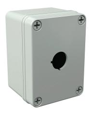
AttaBox Commander series pushbutton enclosure, 1 hole, 22mm, NEMA 1/3R/4X/6P/12, 4 x 3 x 2in (HxWxD), wall mount, polycarbonate, light gray, gloss finish, screw cover.
