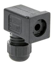
Gefran field wireable connector, 9.4mm DIN 43650 Form C, 90-degree cable entry, 4-pole. For use with Gefran PC series potentiometers.
