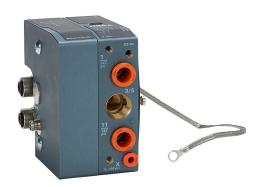
NITRA pneumatic EtherNet/IP protocol modular plate, left supply/ exhaust end, Cv=12.4, (2) 3/8in push-to-connect tubing inlet(s), 3/8in female NPT exhaust(s), 5/32in (4mm) push-to-connect tubing pilot(s), anodized aluminum body, IP65.
