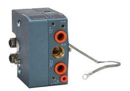
NITRA pneumatic EtherNet/IP protocol modular plate, left supply/ exhaust end, Cv=12.4, (2) 3/8in push-to-connect inlet(s), 3/8in female NPT exhaust(s), 5/32in (4mm) push-to-connect pilot(s), anodized aluminum body, IP65.
