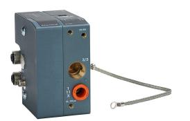
NITRA pneumatic EtherNet/IP protocol modular plate, left supply/ exhaust end, Cv=12.4, 3/8in push-to-connect inlet(s), 3/8in female NPT exhaust(s), anodized aluminum body, IP65.
