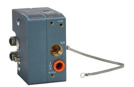
NITRA pneumatic EtherNet/IP protocol modular plate, left supply/ exhaust end, Cv=12.4, 3/8in push-to-connect tubing inlet(s), 3/8in female NPT exhaust(s), anodized aluminum body, IP65.
