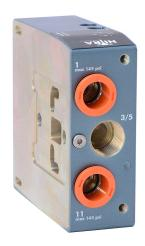
NITRA pneumatic modular plate, right supply/exhaust end, Cv=16.6, (2) 1/2in push-to-connect inlet(s), 3/8in female NPT exhaust(s), anodized aluminum body, IP65.
