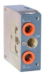
NITRA pneumatic modular plate, right supply/exhaust end, Cv=16.6, (2) 1/2in push-to-connect tubing inlet(s), 3/8in female NPT exhaust(s), anodized aluminum body, IP65.
