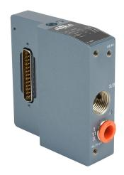
NITRA pneumatic modular plate, left supply/exhaust end, Cv=12.4, 3/8in push-to-connect inlet(s), 3/8in female NPT exhaust(s), anodized aluminum body, IP65.
