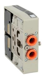
NITRA solenoid valve, compact modular, 5-way, 3-position, center closed, double solenoid, reinforced technopolymer body, IP65, locking manual override, (2) 3/8in push-to-connect outlet(s), Cv=0.5, 24 VDC.
