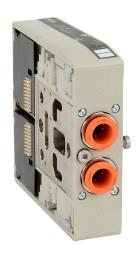
NITRA solenoid valve, compact modular, 5-way, 2-position, double solenoid, reinforced technopolymer body, IP65, locking manual override, (2) 3/8in push-to-connect outlet(s), Cv=1.2, 24 VDC.
