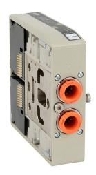
NITRA solenoid valve, compact modular, 5-way, 2-position, double solenoid, reinforced technopolymer body, IP65, locking manual override, (2) 3/8in PTC tubing outlet(s), Cv=1.2, 24 VDC.
