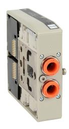
NITRA solenoid valve, compact modular, 5-way, 2-position, single solenoid spring return, reinforced technopolymer body, IP65, locking manual override, (2) 3/8in push-to-connect outlet(s), Cv=1.2, 24 VDC.
