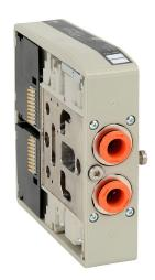
NITRA solenoid valve, compact modular, 5-way, 2-position, single solenoid spring return, reinforced technopolymer body, IP65, locking manual override, (2) 5/16in (8mm) PTC tubing outlet(s), Cv=1, 24 VDC.
