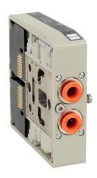
NITRA solenoid valve, compact modular, 5-way, 2-position, single solenoid spring return, reinforced technopolymer body, IP65, locking manual override, (2) 5/16in (8mm) push-to-connect outlet(s), Cv=1, 24 VDC.
