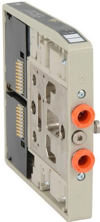
NITRA solenoid valve, compact modular, 5-way, 2-position, single solenoid spring return, reinforced technopolymer body, IP65, locking manual override, (2) 1/4in PTC tubing outlet(s), Cv=0.5, 24 VDC.
