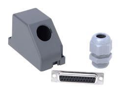
NITRA connector, 25-pin female D-sub, 45-degree cable entry, 22-18 AWG, accepts cable diameter size 0.19-0.39in, IP65. For use with CMV series solenoid valves.
