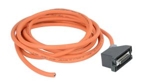
NITRA solenoid valve cable, 25-pin female D-sub to pigtail, 45-degree cable entry, 28 AWG, IP65, 16.4ft/5m cable length. For use with CMV series solenoid valves.
