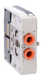
NITRA solenoid valve, double compact modular, 3-way, 2-position, (1) N.C. / (1) N.O., single solenoid spring return, reinforced technopolymer body, IP65, locking manual override, (2) 3/8in push-to-connect outlet(s), Cv=1.2, 24 VDC.
