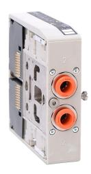
NITRA solenoid valve, double compact modular, 3-way, 2-position, (1) N.C. / (1) N.O., single solenoid spring return, reinforced technopolymer body, IP65, locking manual override, (2) 5/16in (8mm) push-to-connect outlet(s), Cv=1, 24 VDC.
