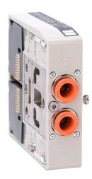
NITRA solenoid valve, double compact modular, 3-way, 2-position, (2) N.O., single solenoid spring return, reinforced technopolymer body, IP65, locking manual override, (2) 3/8in push-to-connect outlet(s), Cv=1.2, 24 VDC.
