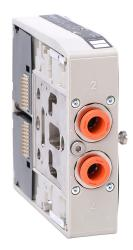
NITRA solenoid valve, double compact modular, 3-way, 2-position, (2) N.O., single solenoid spring return, reinforced technopolymer body, IP65, locking manual override, (2) 5/16in (8mm) push-to-connect outlet(s), Cv=1, 24 VDC.
