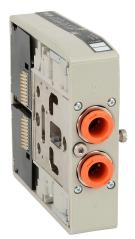
NITRA solenoid valve, double compact modular, 3-way, 2-position, (2) N.C., single solenoid spring return, reinforced technopolymer body, IP65, locking manual override, (2) 3/8in push-to-connect outlet(s), Cv=1.2, 24 VDC.
