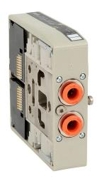
NITRA solenoid valve, double compact modular, 3-way, 2-position, (2) N.C., single solenoid spring return, reinforced technopolymer body, IP65, locking manual override, (2) 5/16in (8mm) push-to-connect outlet(s), Cv=1, 24 VDC.
