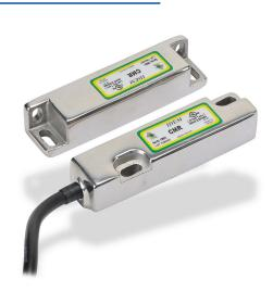
IDEM safety switch set, non-contact magnetic, (1) N.C. safety output(s), (1) N.O. monitoring output(s), 316 stainless steel housing, 83 x 20mm, pigtail, 32.8ft/10m cable length.
