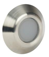
Captron LED indicating light, permanent light function, IP69K, 22mm, red/yellow/green/blue/white/orange/violet, 40mm, round, plastic base, stainless steel bezel, 24 VDC, full voltage. Requires M8 4-pole connection cable.
