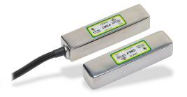
IDEM safety switch set, non-contact coded magnetic, rear mount, (2) N.C. safety output(s), (1) N.O. monitoring output(s), 316 stainless steel housing, 83 x 20mm, pigtail, 16.4ft/5m cable length.
