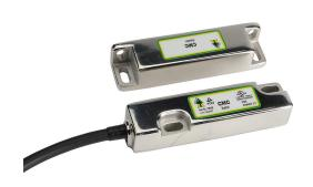
IDEM safety switch set, non-contact coded magnetic, (2) N.C. safety output(s), (1) N.O. monitoring output(s), 316 stainless steel housing, 83 x 20mm, 8-pin M12 quick-disconnect, 9.8in/250mm cable length.
