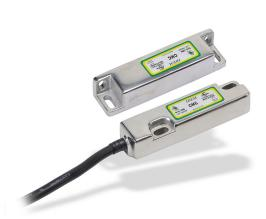
IDEM safety switch set, non-contact coded magnetic, (2) N.C. safety output(s), (1) N.O. monitoring output(s), 316 stainless steel housing, 83 x 20mm, pigtail, 16.4ft/5m cable length.
